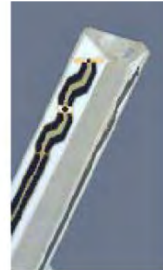
Figure 2.3 Probe Thick-Film Technique
