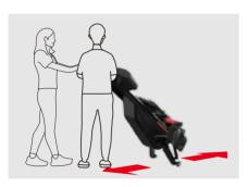
2 Use the transportation wheels on the front stabilizer to transport the rower to the desired location. Always hold the rear stabilizer during the entire movement.
