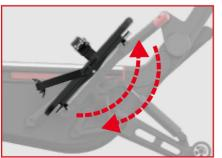
open the lock buckle, hold and move it to left (right) to quickly release the straps. Through the supportive gas spring at the bottom of the foot pedal, the motion posture of the foot can be adaptively raised or lowered.
