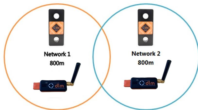
**Example 2:** Using two TD-3.0 with two TL-3.0 Telemetry Tensile links outside of the range of each other.
