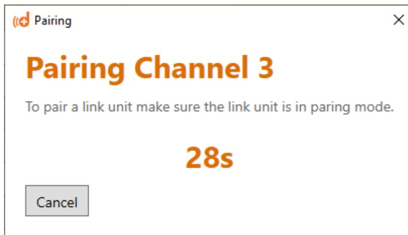
If the timer reaches zero before the products are paired than the pair cycle must be restarted.
