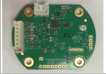
RF circuitry with can removed
