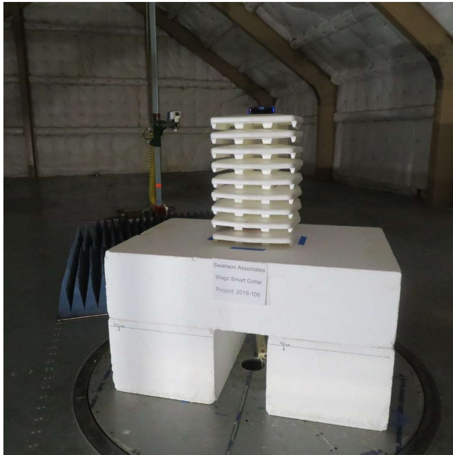
EUT set up in OATS, 18-25GHz EUT on 1.5m polystyrene stand
