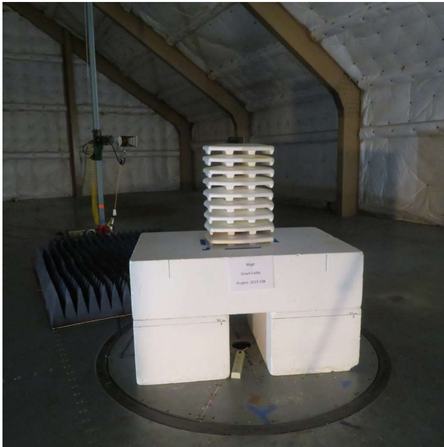
EUT set up in OATS, 1-18GHz EUT on 1.5m polystyrene stand
