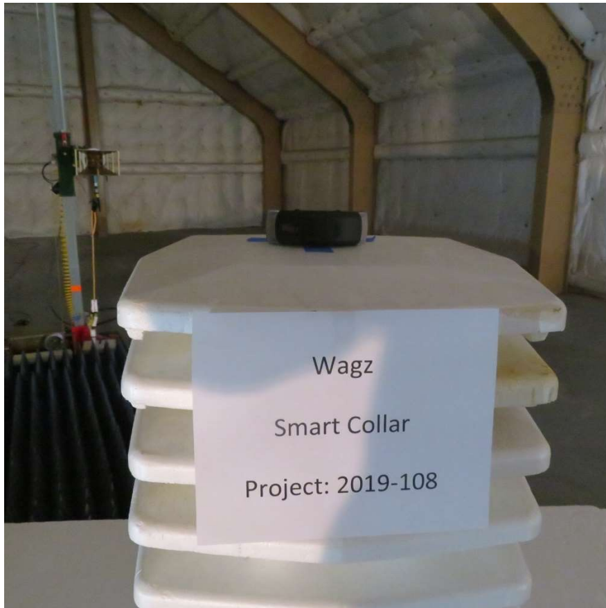
EUT set up in OATS Worst case orientation, front
