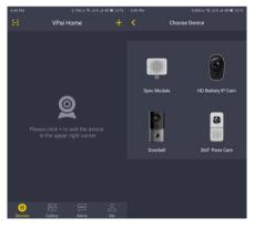
Connect the Sync Module to the power supply. Tap "Start Config" button when the red LED light on the sync module starts flashing, and after hearing the "pairing mode".
