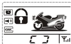
once. If moving of object or somebody is detected for 15 second by microwave sensor,then the engine will be cut off,the flash lights will gleam,the siren will chirp loudly for 30 secondsto remind and warn the car owner. The transmitter will remit a sound like Bi Bi Bi for 30 seconds, at the same time the icon of headlight and background light will light on, and the transmitter vibrates for 8 times.
