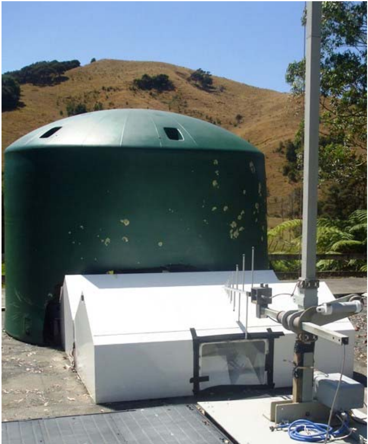
Test shed showing the use of a log periodic antenna 300 – 1000 MHz
