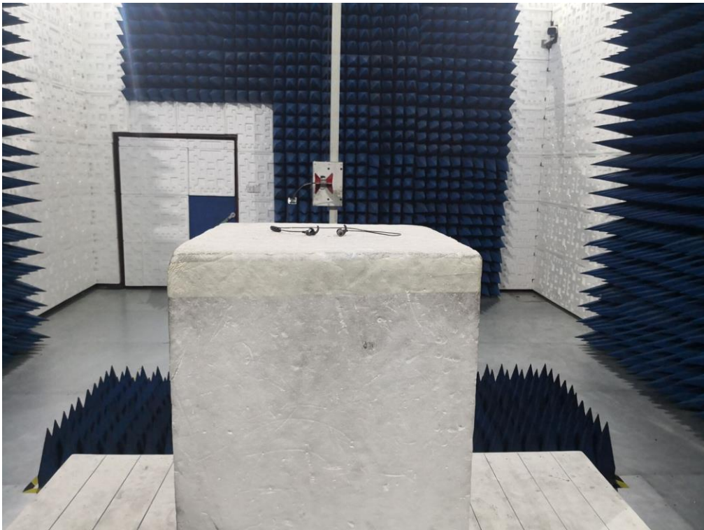
RADIATED EMISSION TEST SETUP ABOVE 1GHZ
