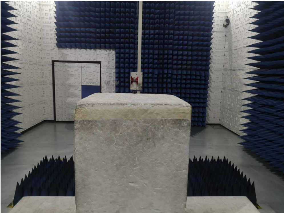
RADIATED EMISSION TEST SETUP ABOVE 1GHz
