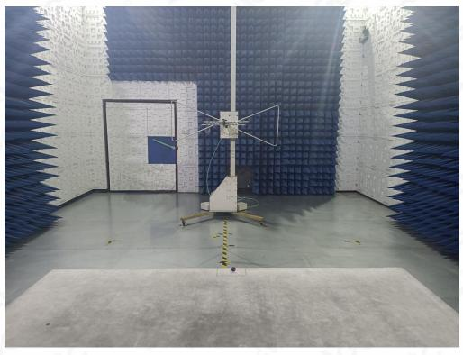
RADIATED EMISSION TEST SETUP ABOVE 1GHz
