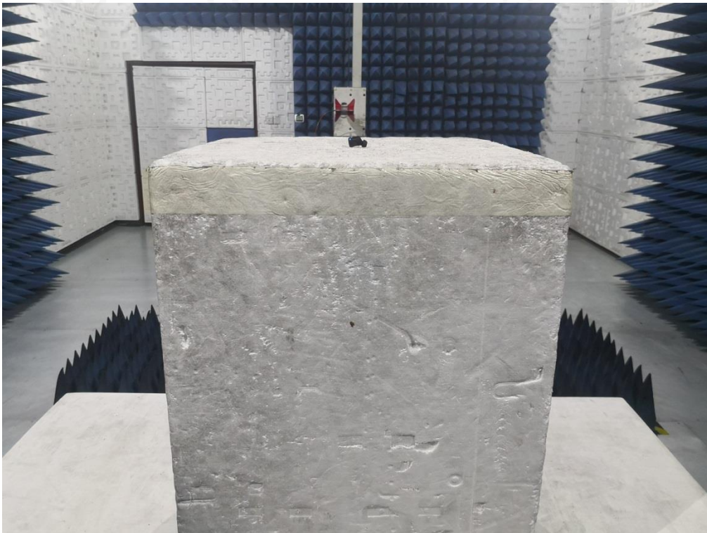
RADIATED EMISSION TEST SETUP ABOVE 1GHZ
