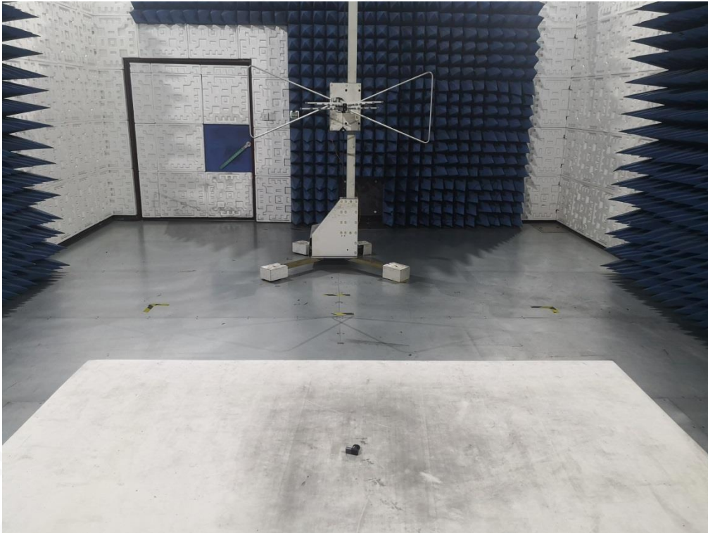
RADIATED EMISSION TEST SETUP ABOVE 1GHZ
