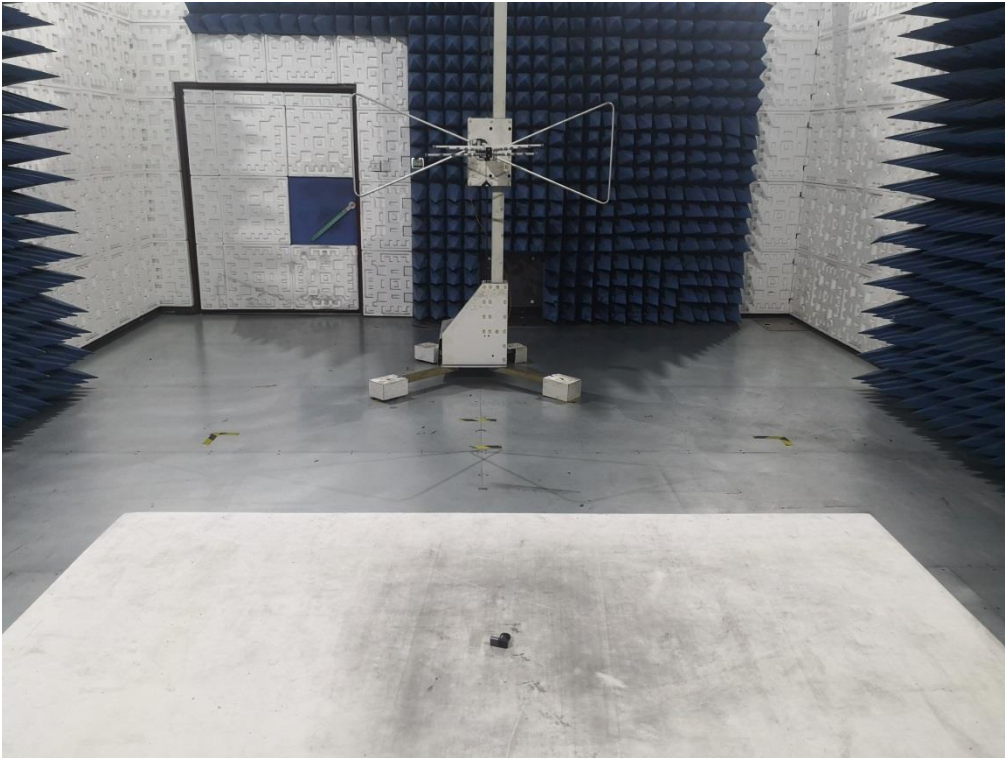
RADIATED EMISSION TEST SETUP ABOVE 1GHz
