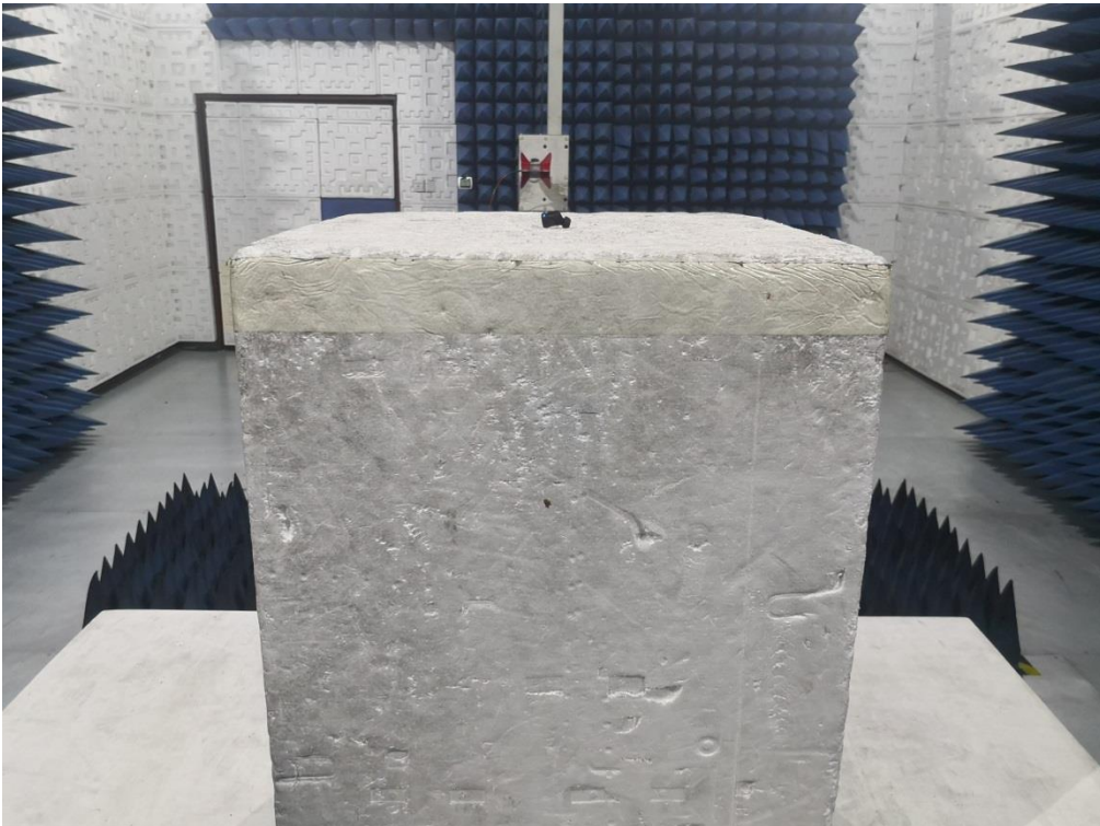
RADIATED EMISSION TEST SETUP ABOVE 1GHz
