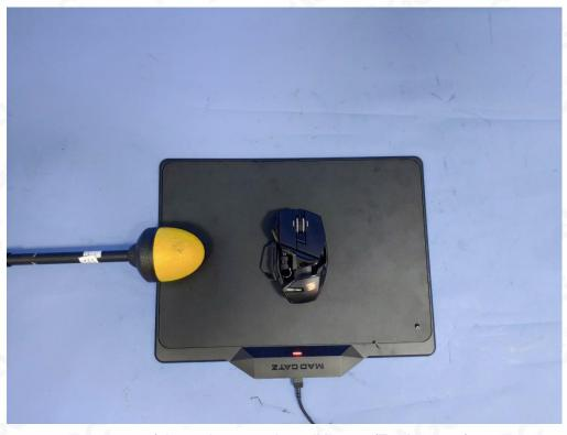
center of the probe away the coil is 5 cm(Top is 10 cm)
