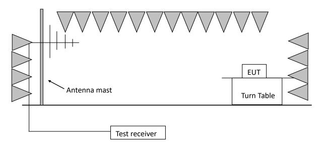
Note: This test configuration is used for above 30MHz, when measure the result of below 30MHz please refer section 4.2 test configuration.
