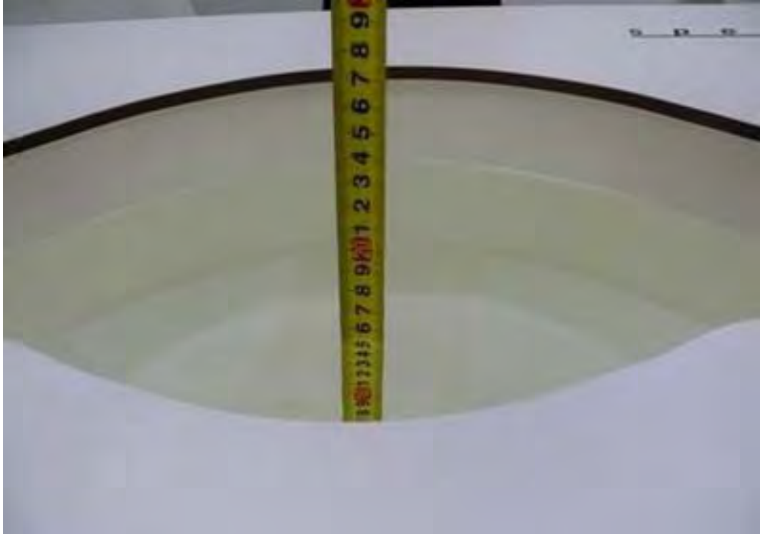
Picture 3: Liquid depth in the flat Phantom
