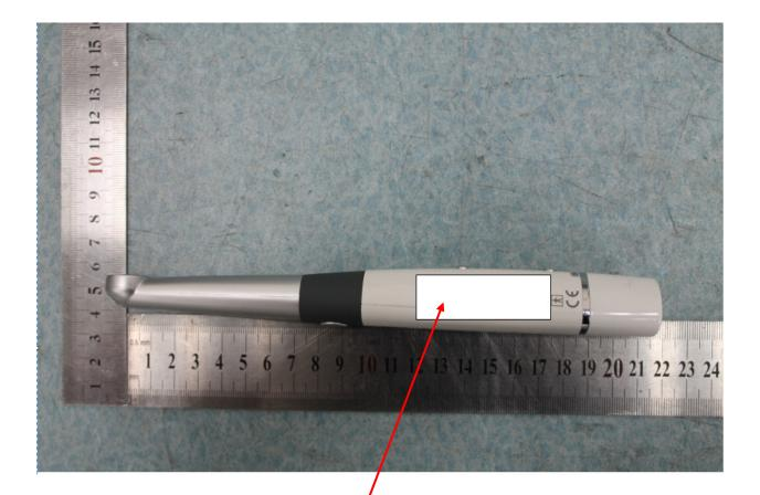
Product label with FCC ID: 2ASFG-CS1500H and IC: 24914-CS1500H will be laser printed at this place. The statement according to FCC part 15 §15.19(a)(3) has been added in CS 1500 Safety & Regulatory Guide, page 22.
