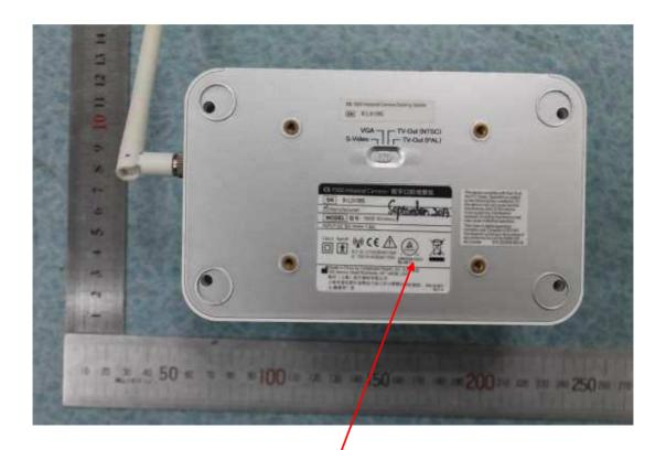
Product label with FCC ID: 2ASFG-CS1500D and IC: 24914-CS1500D will be located at this place. The statement according to FCC part 15 §15.19(a)(3) has been added in CS 1500 Safety & Regulatory Guide, page 22.
