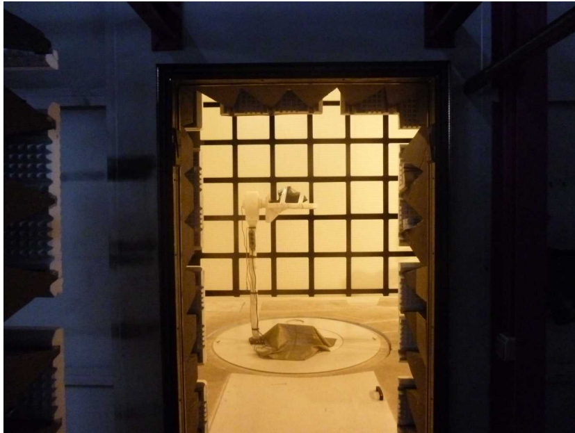
Photo 1: EUT at the anechoic chamber
