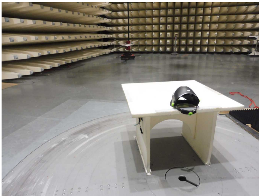
Photo 10: EUT at the semi-anechoic chamber
