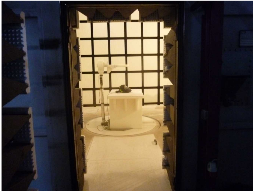
Photo 7: EUT at the anechoic chamber, loop antenna test setup
