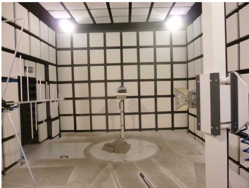
Photo 6: EUT at the anechoic chamber
