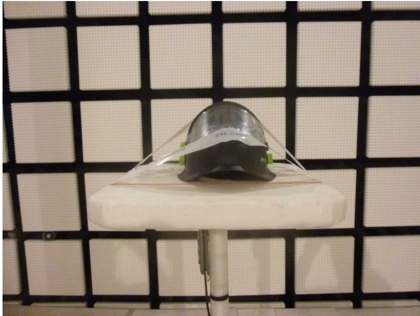
Photo 5: EUT at the anechoic chamber
