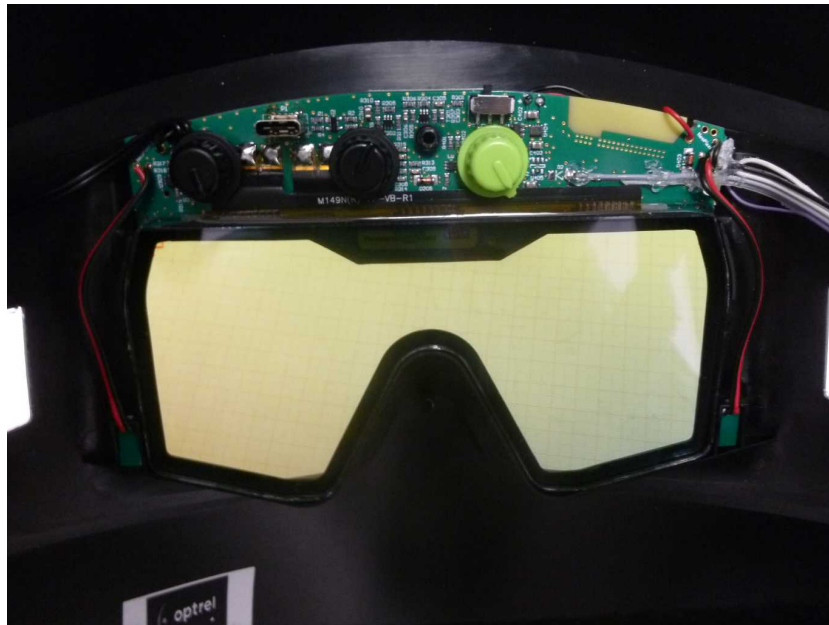
Photo 1: PCB front side view, inside the helmet
