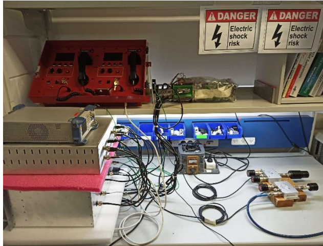
Photograph No.1 Peak output power, OBW, emission mask measurement setup
