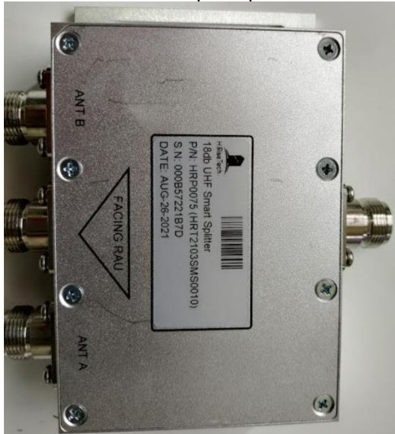
Photograph No.6 18dB Smart splitter top view
