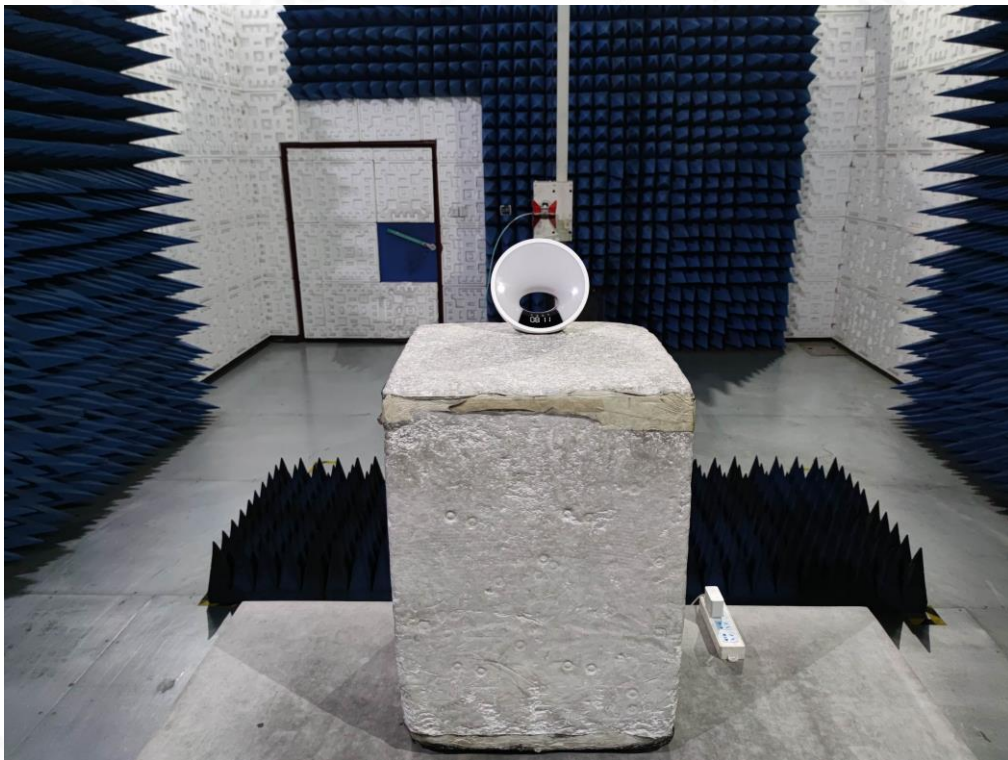
RADIATED EMISSION TEST SETUP ABOVE 1GHZ
