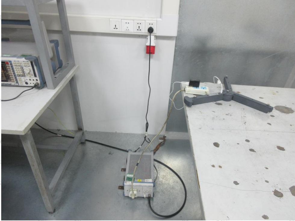
Photo of Conducted Emission Measurement
