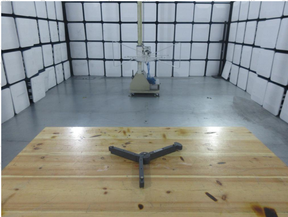
Photo of Radiation Emission Test
