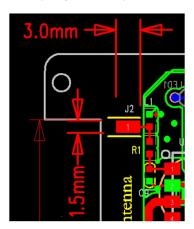
Spring antenna location on PCB are J2, and the Empty Area except spring antenna should be see just follow the below two charts.
