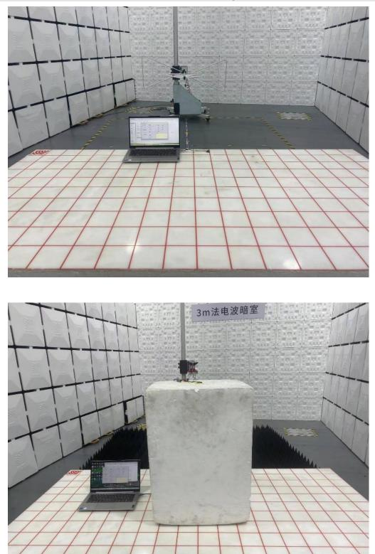
Radiated Emissions and Band Edge Measurement
