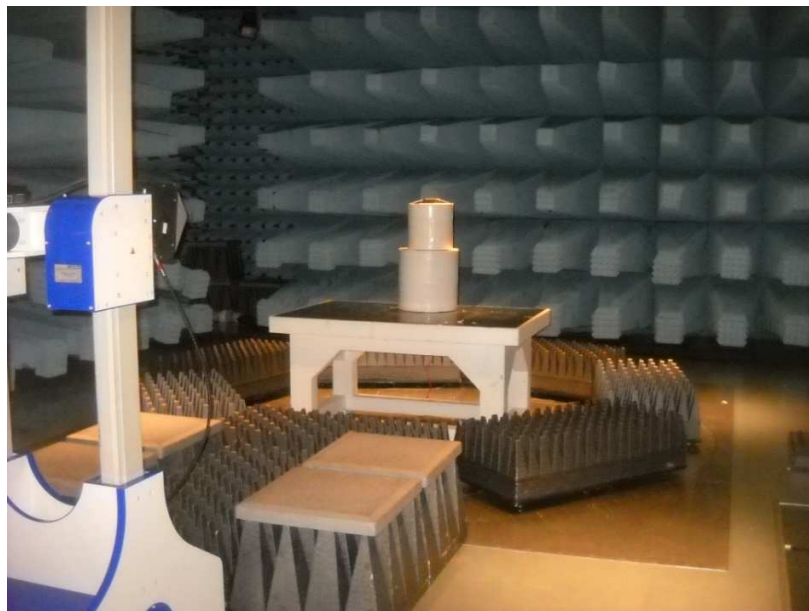
Radiated emissions set-up for frequencies above 1 GHz
