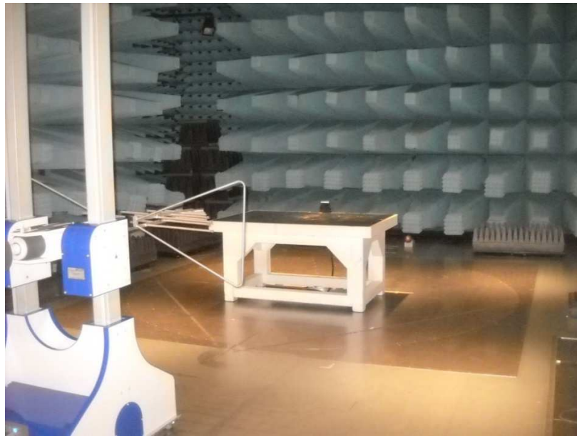
Radiated emissions set-up for frequencies below 1 GHz
