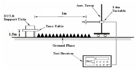
The radiated emission Below 1GHz tests were performed in the 3 meters chamber test site A , above 1GHz tests were performed in the 3 meters chamber test site B, using the setup accordance with the ANSI C63.10-2013. The specification used was the FCC 15.209, and FCC 15.407 limits and RSS-247, RSS-Gen limits.
