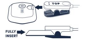
PRESS AND HOLD the button for 2 SECONDS. The light will blink BLUE 10 TIMES after the device has powered on. (Note: the device may take up to 15 seconds to power on)
