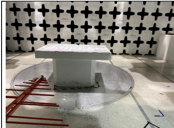
Radiated Emission Test below 1GHz Front View
