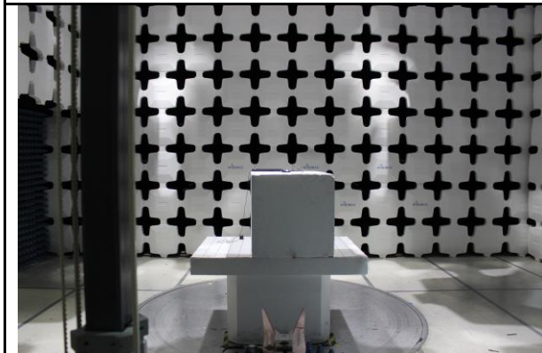
Radiated Emission Test Above 1GHz Front View
