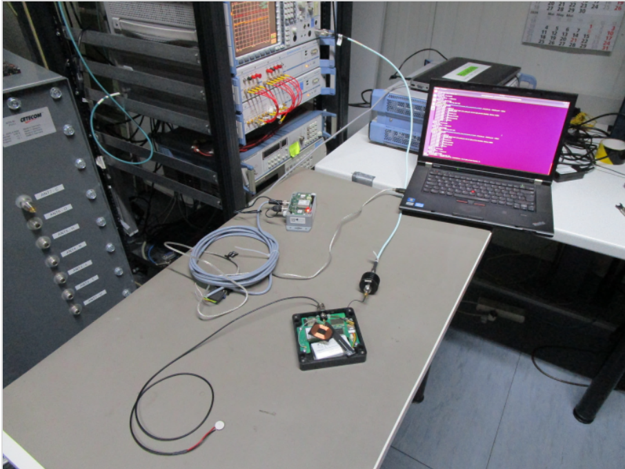
Photograph 5: EUT Test Setup conducted Measurements in the radio lab
