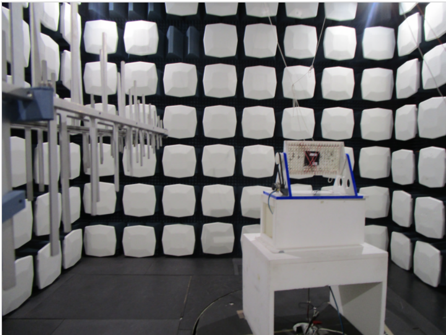
Photograph 2: Overall view of the EUT Test Setup in the fully anechoic chamber, Radiated interference field strength
