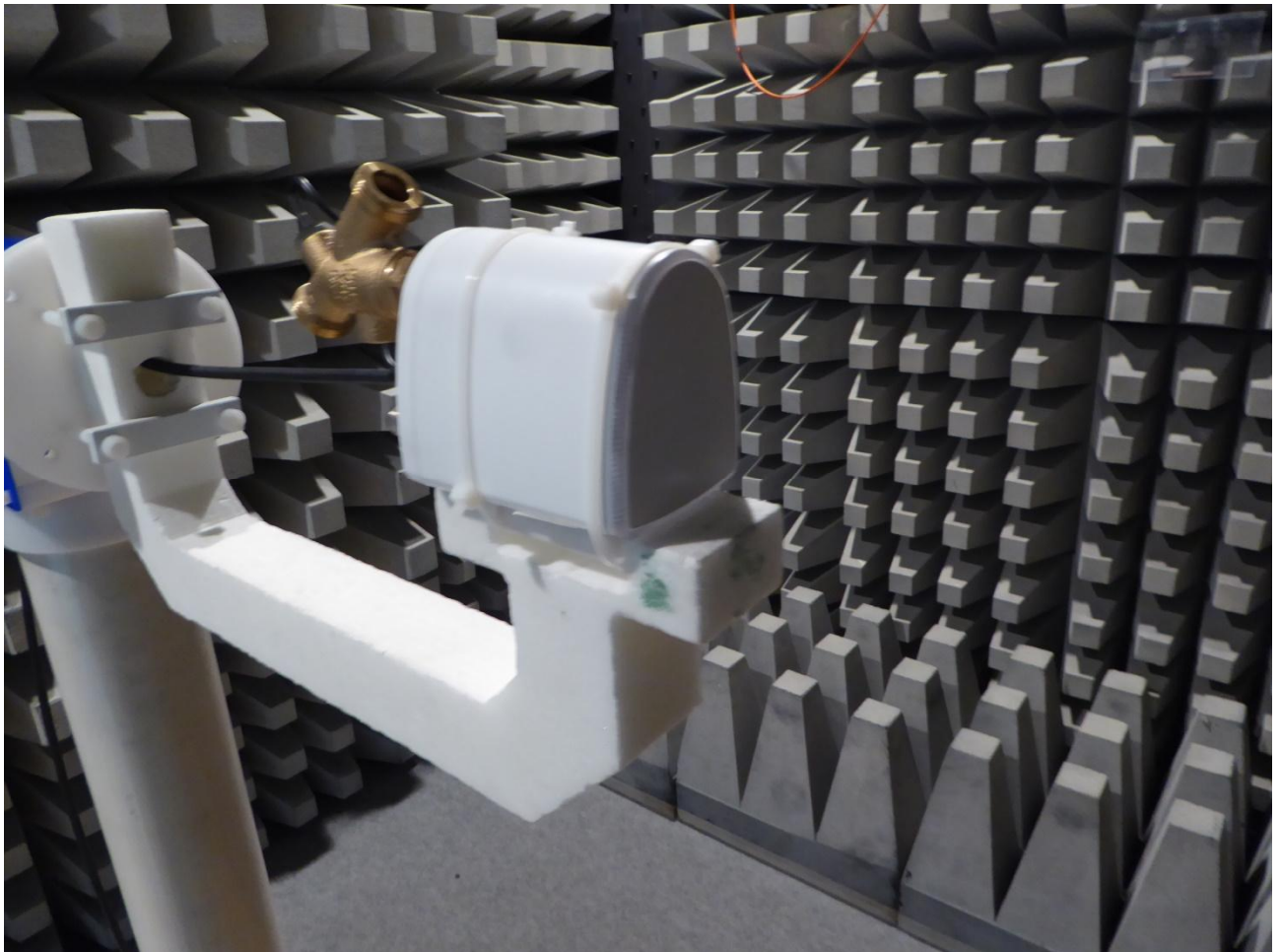
Test setup fully anechoic chamber
