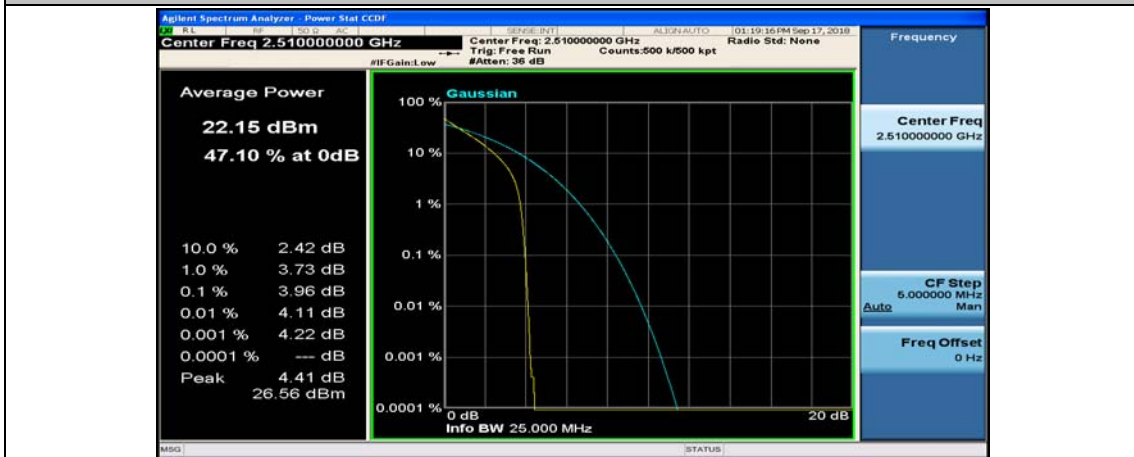
(Channel Bandwidth:20 MHz)_LCH_QPSK_100RB#0
