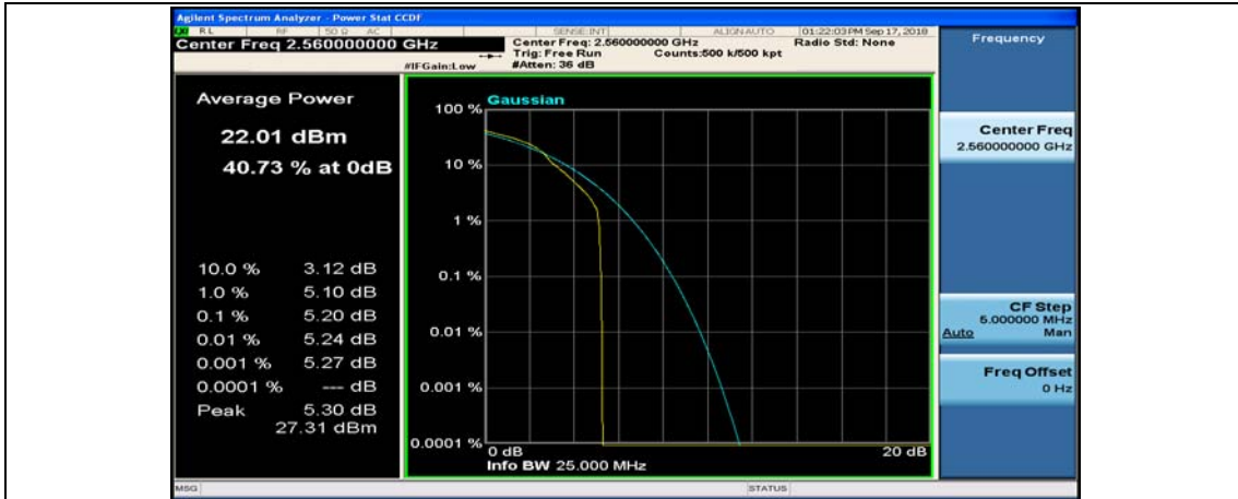
(Channel Bandwidth:20 MHz)_HCH_16QAM_1RB#99
