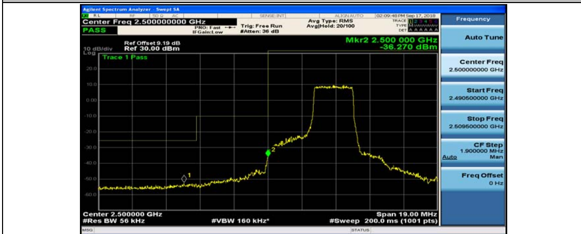
(Channel Bandwidth: 5 MHz)_LCH_QPSK_25RB#0
