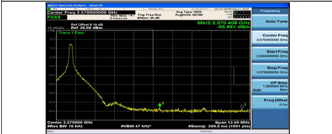
Channel Bandwidth: 10 MHz_HCH_16QAM_1RB#49
