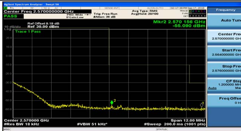
(Channel Bandwidth:15 MHz)_HCH_QPSK_1RB#74
