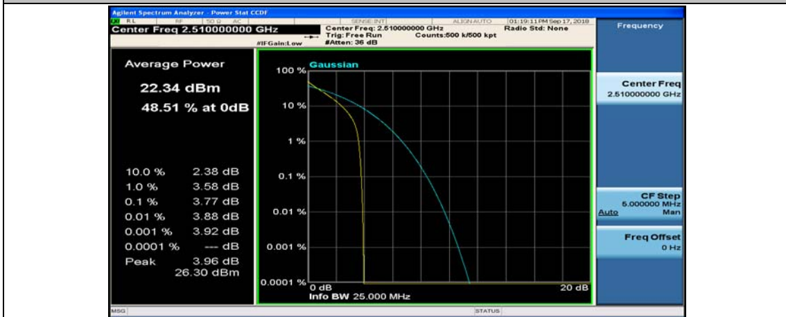
(Channel Bandwidth:20 MHz)_LCH_QPSK_50RB#50
