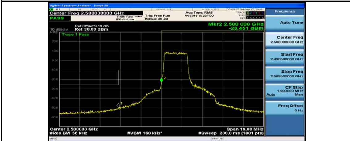
(Channel Bandwidth: 5 MHz)_LCH_16QAM_12RB#6
