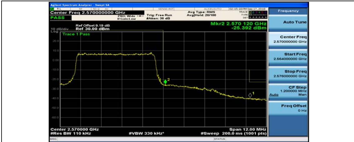
Channel Bandwidth: 10 MHz_HCH_16QAM_50RB#0
