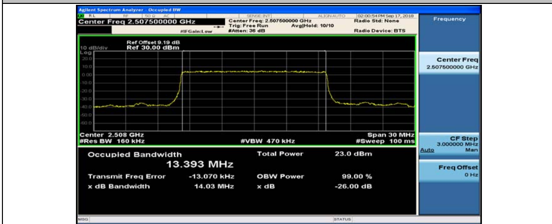
(Channel Bandwidth:15 MHz)_LCH_16QAM_75RB#0
