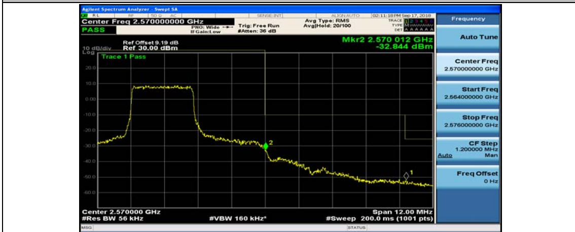
(Channel Bandwidth: 5 MHz)_HCH_QPSK_12RB#6
