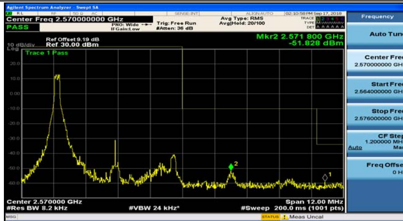
(Channel Bandwidth: 5 MHz)_HCH_16QAM_1RB#12
