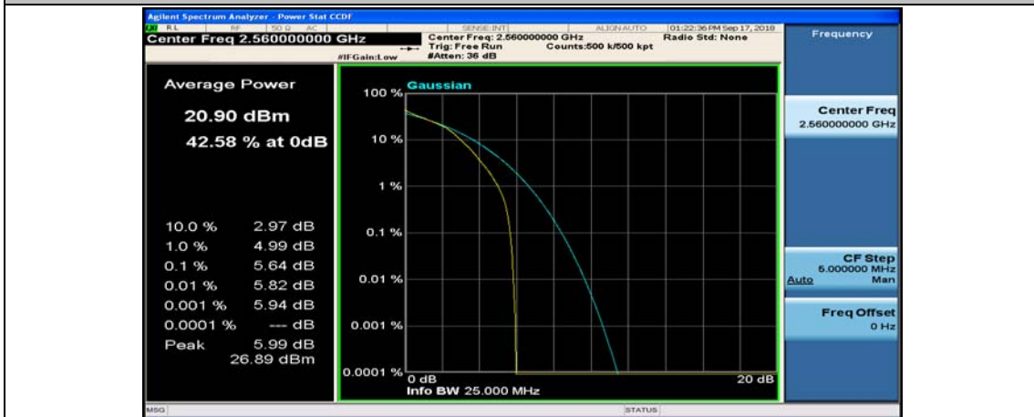
(Channel Bandwidth:20 MHz)_HCH_16QAM_50RB#25
