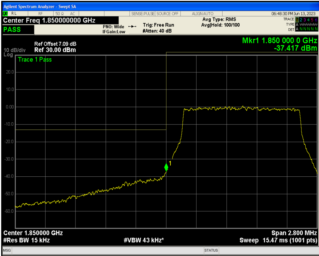
Band2 QPSK BW=1.4MHz Channel=19193 RB Size=6 Position=#0
