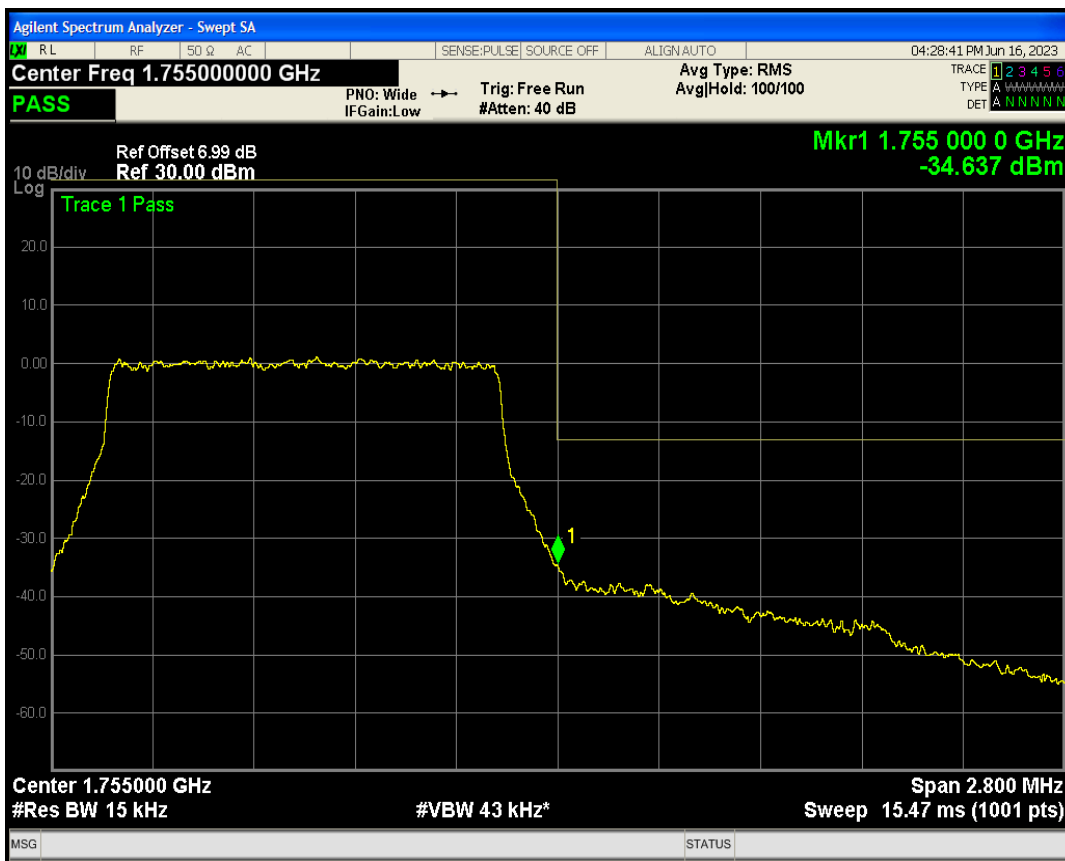
Band4 QAM16 BW=5MHz Channel=20375 RB Size=25 Position=#0
