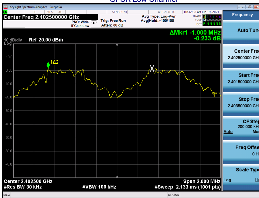
Test plots GFSK Low Channel
