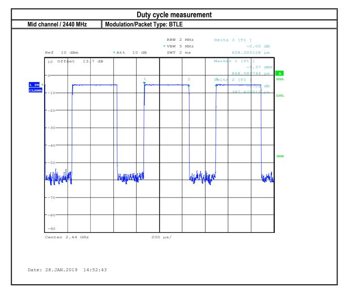
Duty cycle =61.7% Duty cycle correction factor =10\*log (1/0.617) = 2.09 dB
