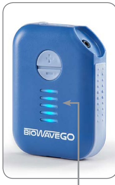
LED Bar Graph Indicator Displaying Signal Intensity
