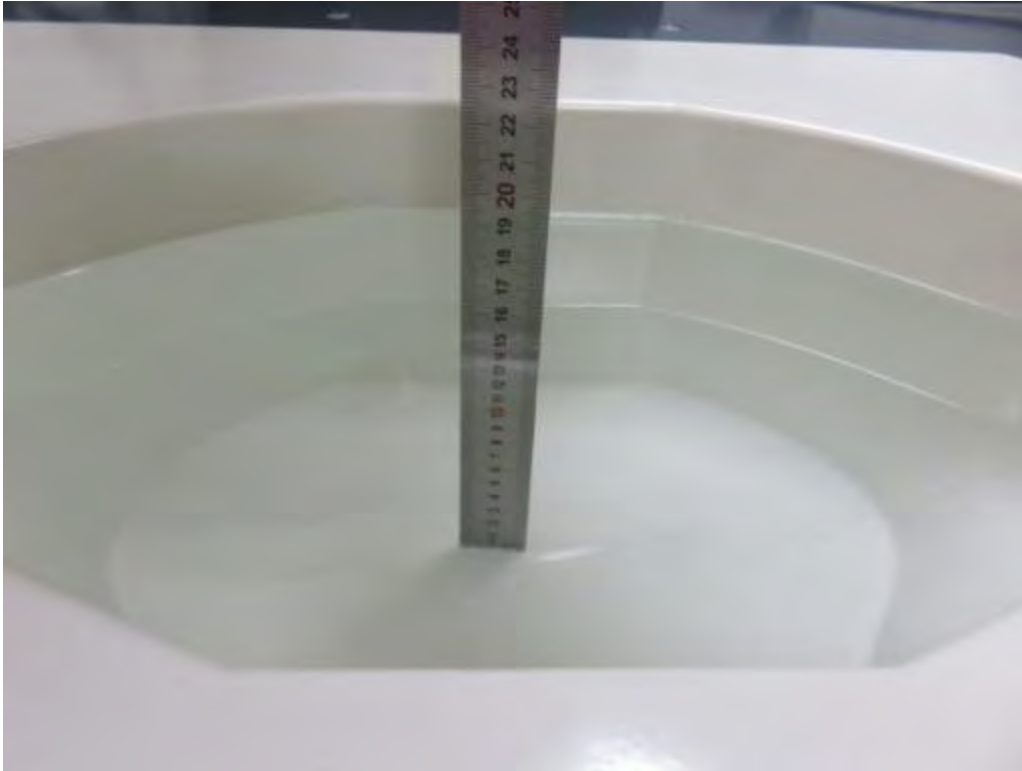
Photograph of the depth in the Body Phantom (835MHz, 15.3cm depth)
