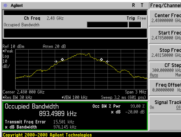
20dB Bandwidth plot on channel 78 (1Mbps)
