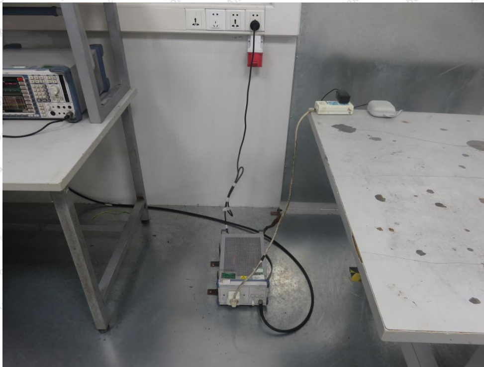
Photo of Power Line Conducted Emission Test
