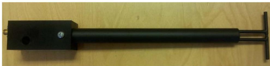
Figure 1 – MVG COMOSAR Validation Dipole
