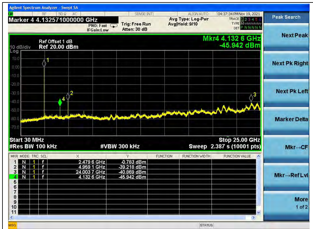
(30MHz to 25GHz, Channel 78, \pi/4 -DQPSK)
