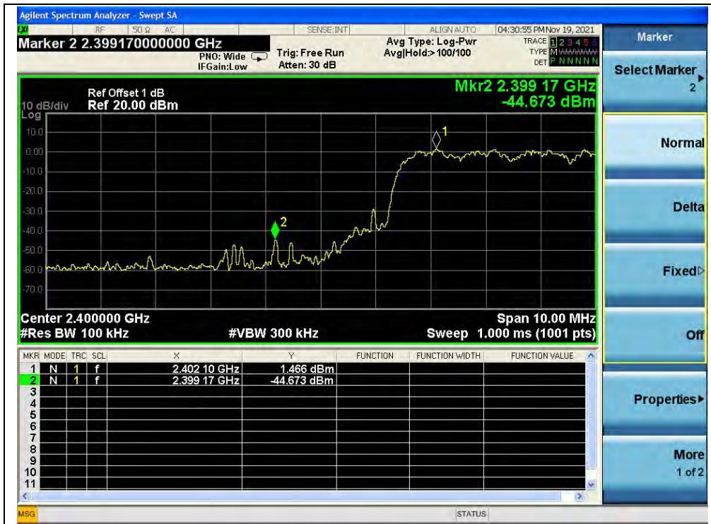
(Band edge with hopping on, Channel 0, 8-DPSK)
