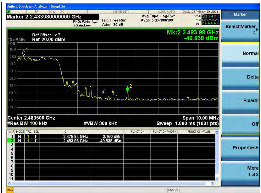
(Band edge with hopping on, Channel 78, 8-DPSK)
