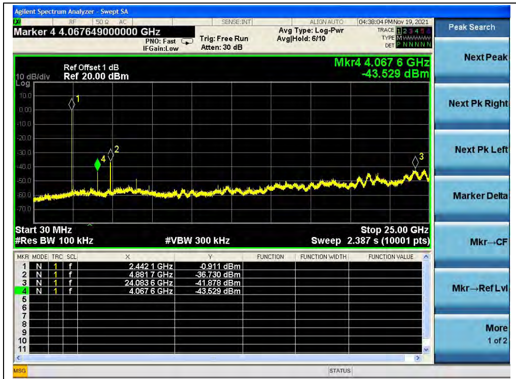
(30MHz to 25GHz, Channel 39, \pi/4 -DQPSK)
