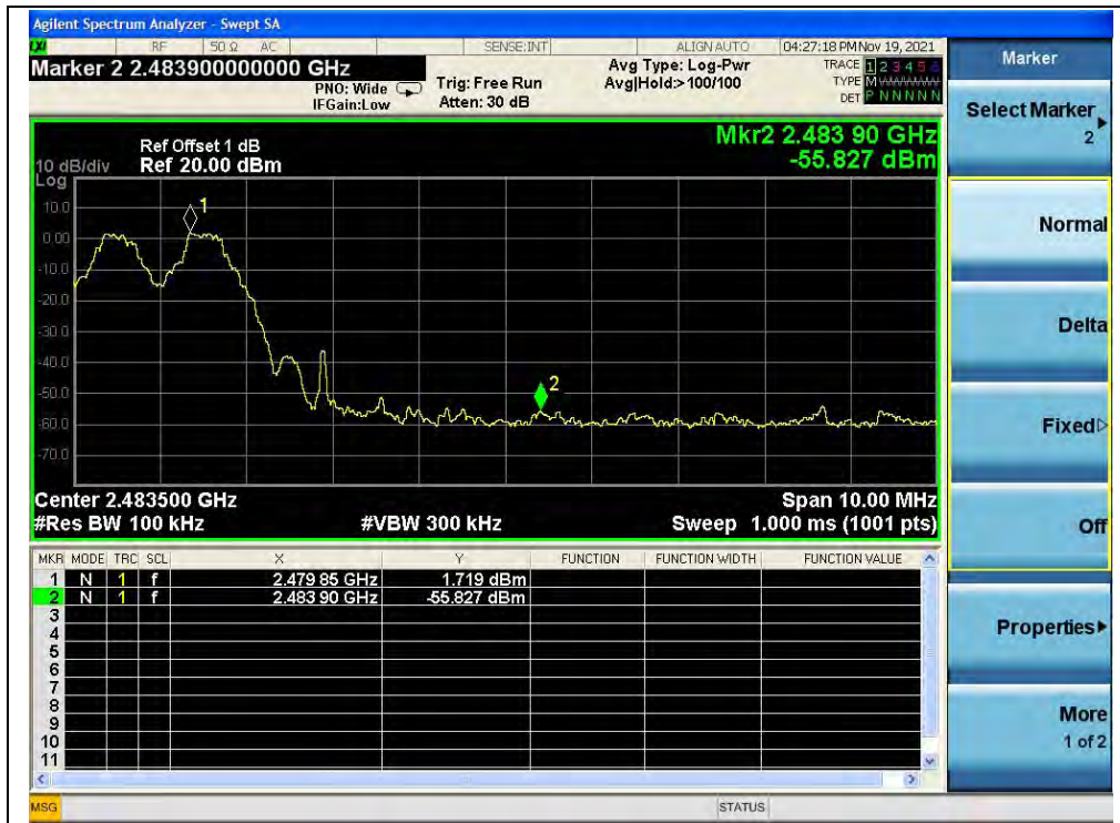
(Band edge with hopping on, Channel 78, GFSK)
