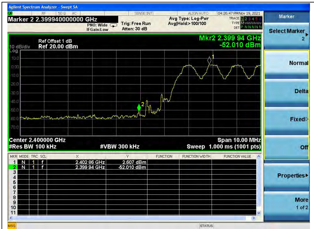
(Band edge with hopping on, Channel 0, GFSK)
