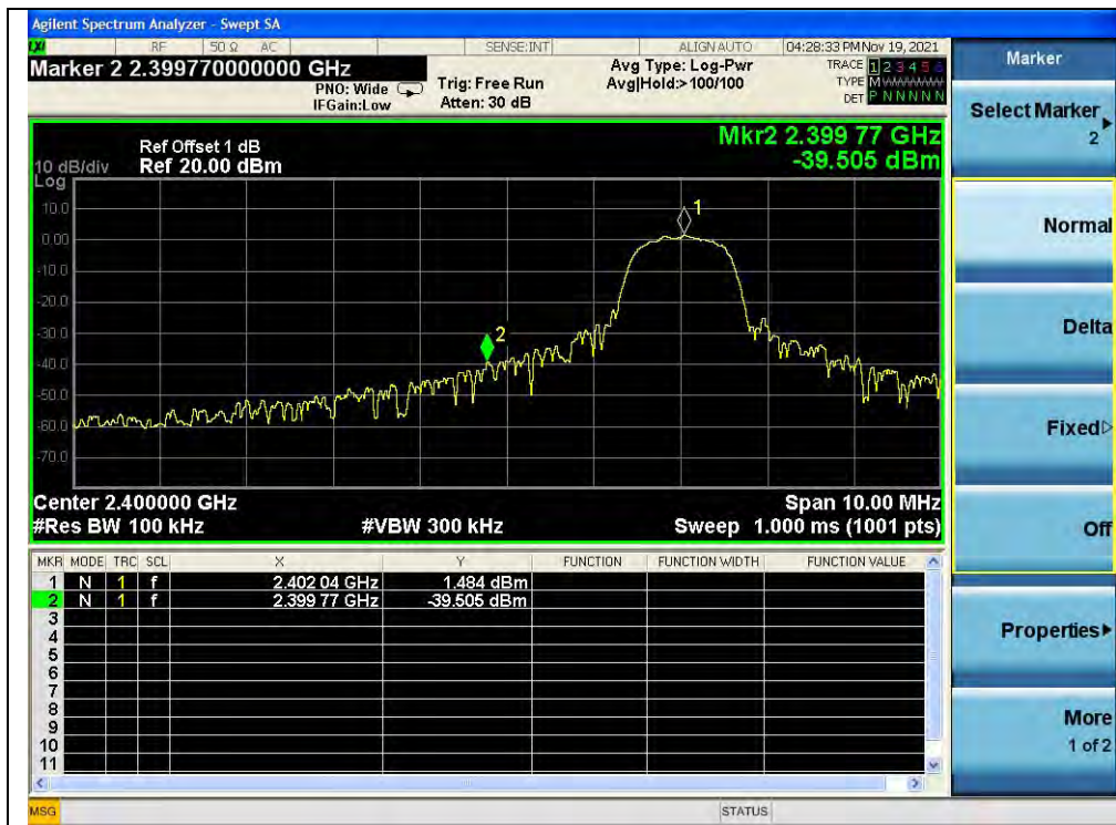
(Band edge, Channel 0, \pi/4 -DQPSK)
