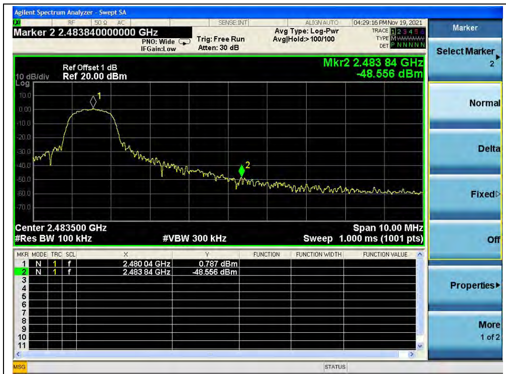
(Band edge, Channel 78, \pi/4 -DQPSK)
