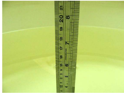
Fig 6.12 Photo of Liquid Height for Body SAR
