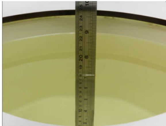
Fig 10.1 Photo of Liquid Height for Body SAR
