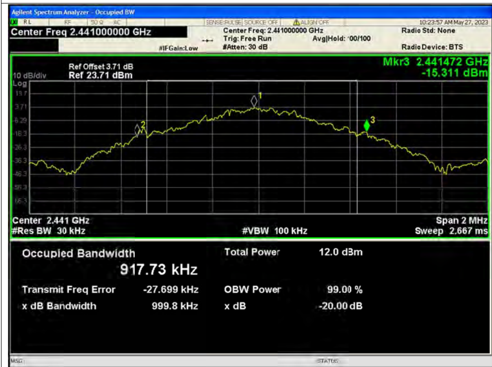
-20dB Bandwidth NVNT 1-DH5 2441MHz Ant1
