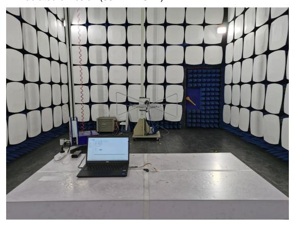
3. Radiated emission (9KHz-30MHz)
