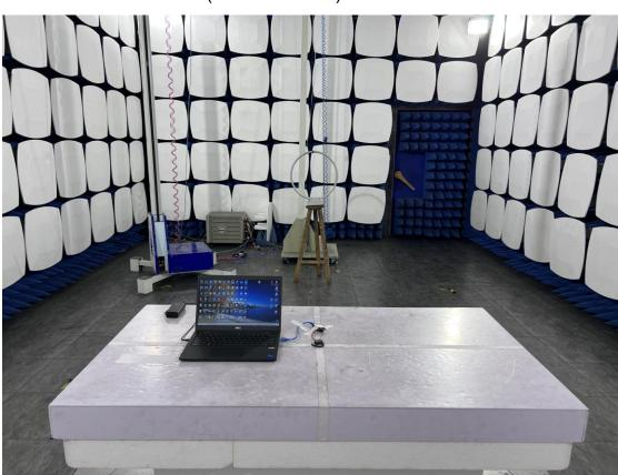
3. Radiated emission (9KHz-30MHz)
