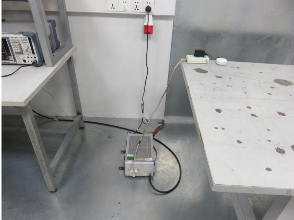
Photo of Conducted Emission Measurement
