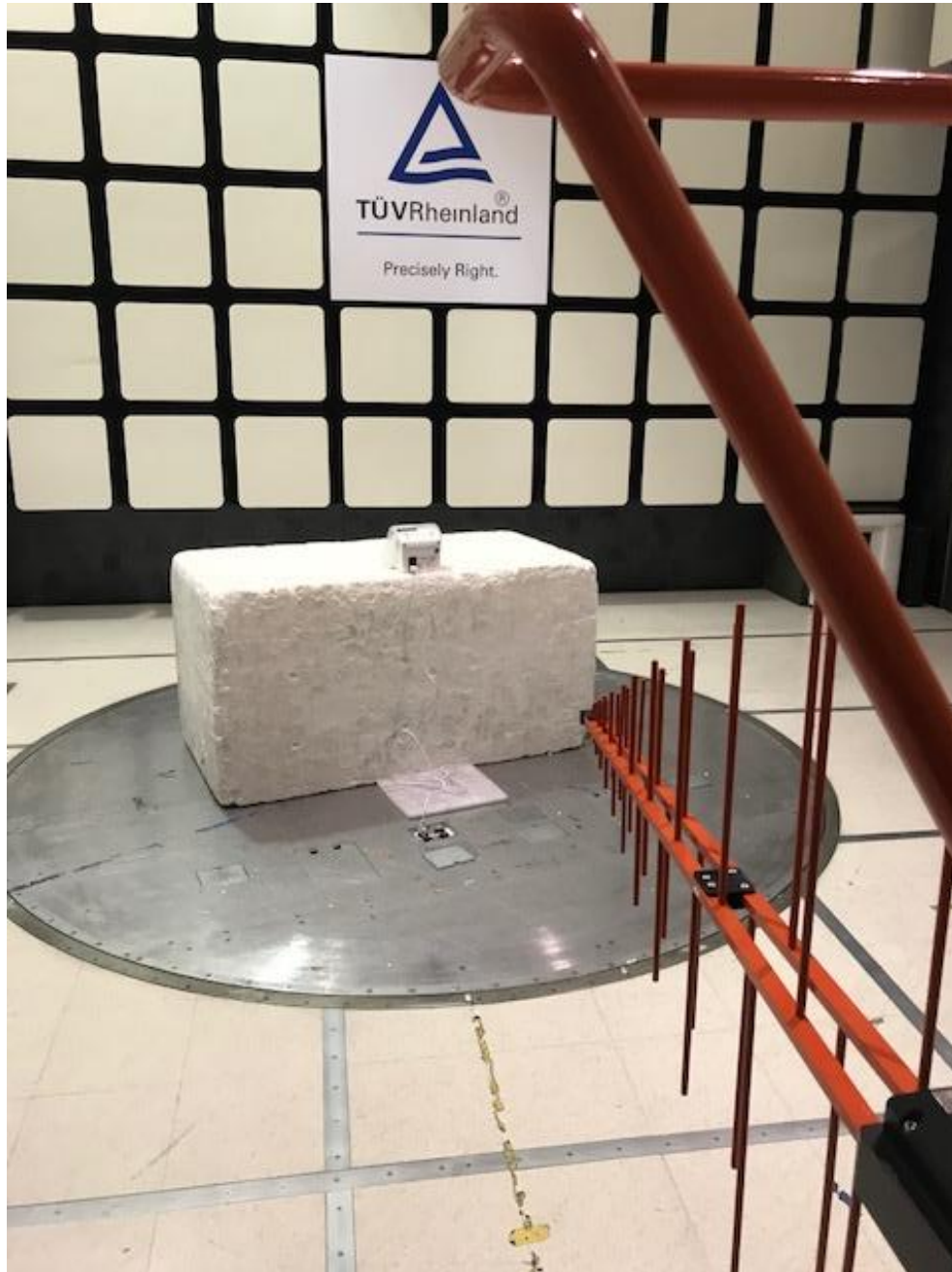
Figure 3 - Radiated Emissions Test Setup 30 - 1000 MHz - Front
