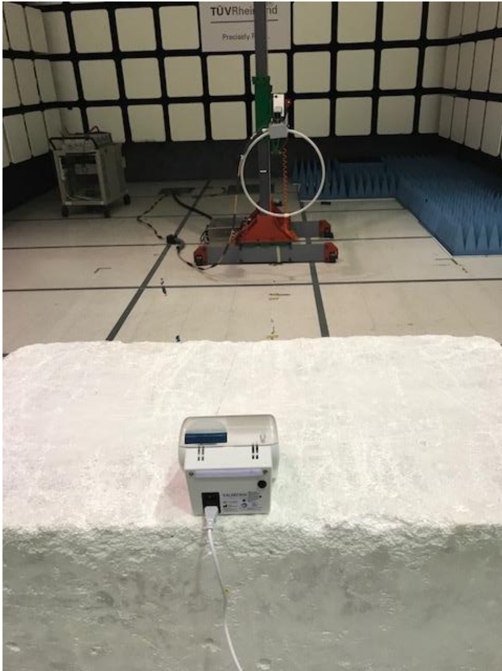
Figure 3 - Radiated Emissions Test Setup 9 kHz-30 MHz - Back
