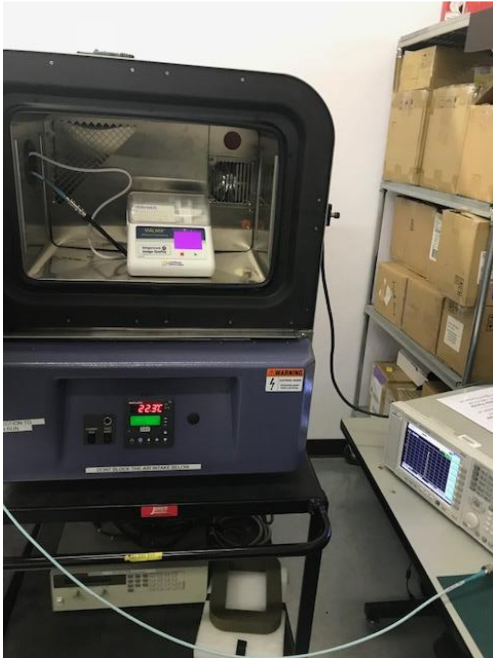
Figure 11 – Frequency Stability test setup
