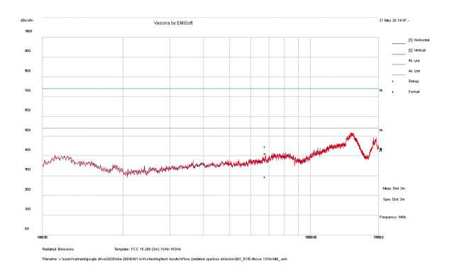
Frequency Raw dBuV AF dB Cable Level Measurement Pol Hgt Azt Limit Margin Pass/Fail Loss dBuV/m dB  $\mathsf{MHz}$ Deg dBuV/m Type cm 6792.35 20.94 19.63 0.82 41.40 ٧ 400 153 74.00 -32.60 Pass Peak Max 6792.35 8.97 19.63 0.82 29.43 ٧ 400 153 54.00 -24.57 Average Max Pass
